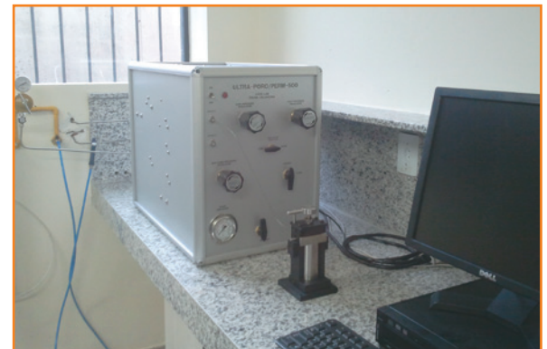
Figure 53 - Permoporosimeter acquired for the Petrophysical Laboratory at Campina Grande Federal University.
