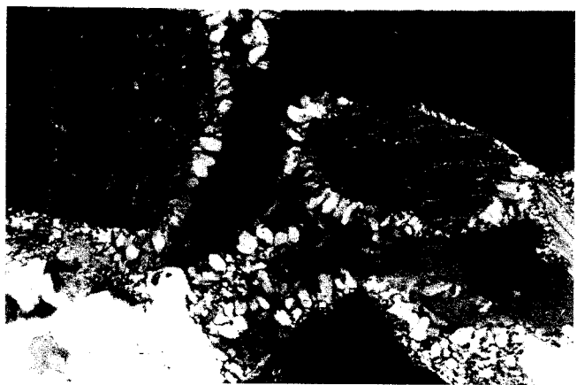
Foto 12 - Detalhe da drusa formada por microquartzo recobrendo os grãos do arcabouço. Poço 12; prof. 2 945,0 m; XN; aumento 70X. Photo 12 - Detail of druse formed by microquartz covering the framework grains. Well 12; depth 2,945.0 m; XN; enlargement 70X.
