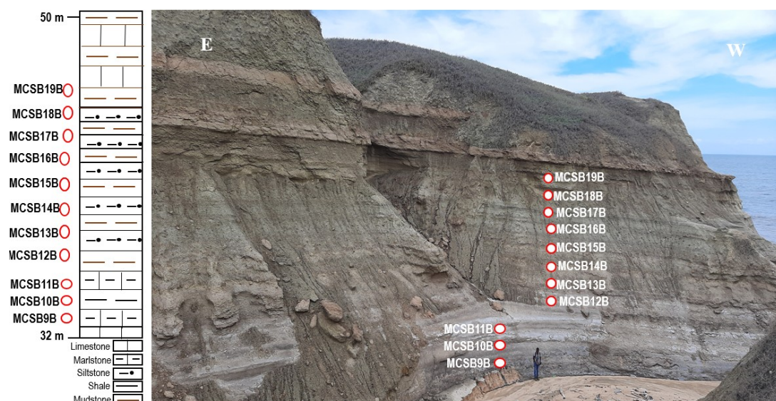
Figure 5. Outcrop ML3. Sedimentological profile of the ML3 outcrop located in the Cabo de São Braz region, Kwanza Basin.
